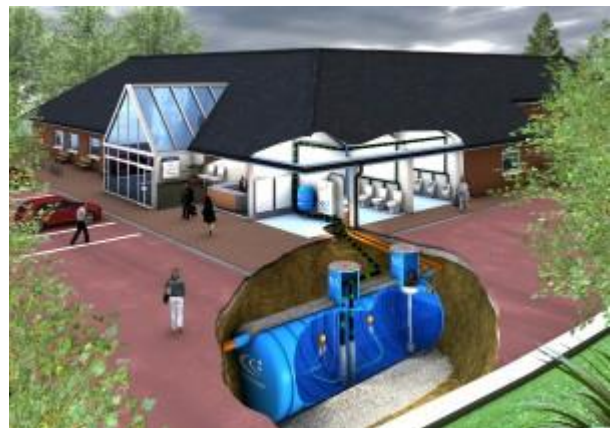
Figure 8: Example of an underground rainwater collection tank.
